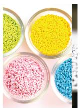
In addition to colours, additives and fillers can also be added to enhance the performance of the base polymer properties such as; UV stability, flame retardancy, anti-slip, anti-block, anti-static, electrical conductivity, density, hardness, scratch resistance, mould release, cycle times, plus many other properties can all be achieved with the right modification.
